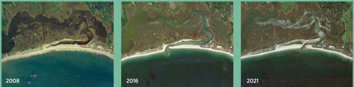
FIGURE 5 Aerial images show how the Allens Pond inlet has changed positions over time. The inlet completely closed in 2008. In 2016, the inlet was almost closed, and it had to be re-opened in early 2017. The inlet closed again in early 2021, and the 2021 image shows the inlet position after it had been opened.
