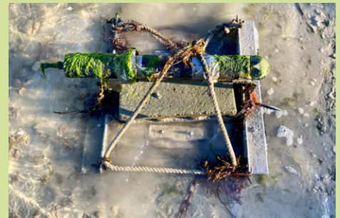
Retrieving a sensor after a months-long deployment in Allens Pond (top) Deployment frame containing a sensor that measured currents and water levels in the Slocums River (bottom)
